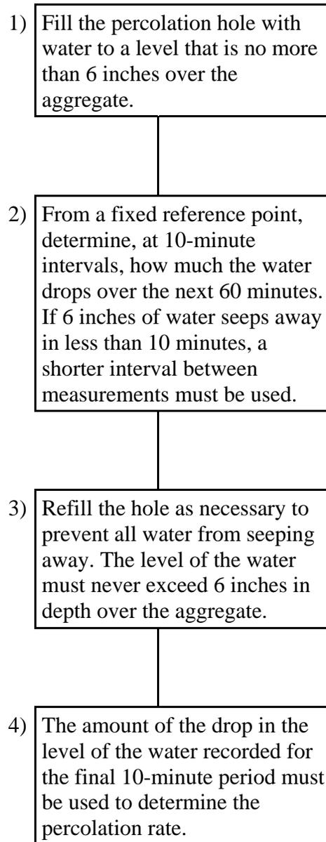
NOTE: The minimum time in which a fast percolation test may be completed is 1 hour. The level of the water must never exceed 6 inches over the aggregate during a fast percolation test.
