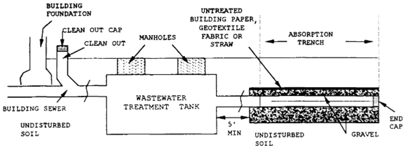
**NAC 444.8354 Absorption trench system: Design criteria. ([NRS 439.200, 444.650](#))**
