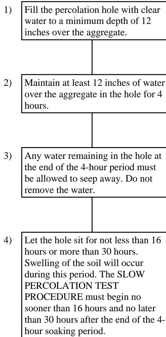
**NAC 444.7968 Slow percolation test procedure. (NRS 439.200, 444.650) The following flow chart illustrates the slow percolation test procedure:**
