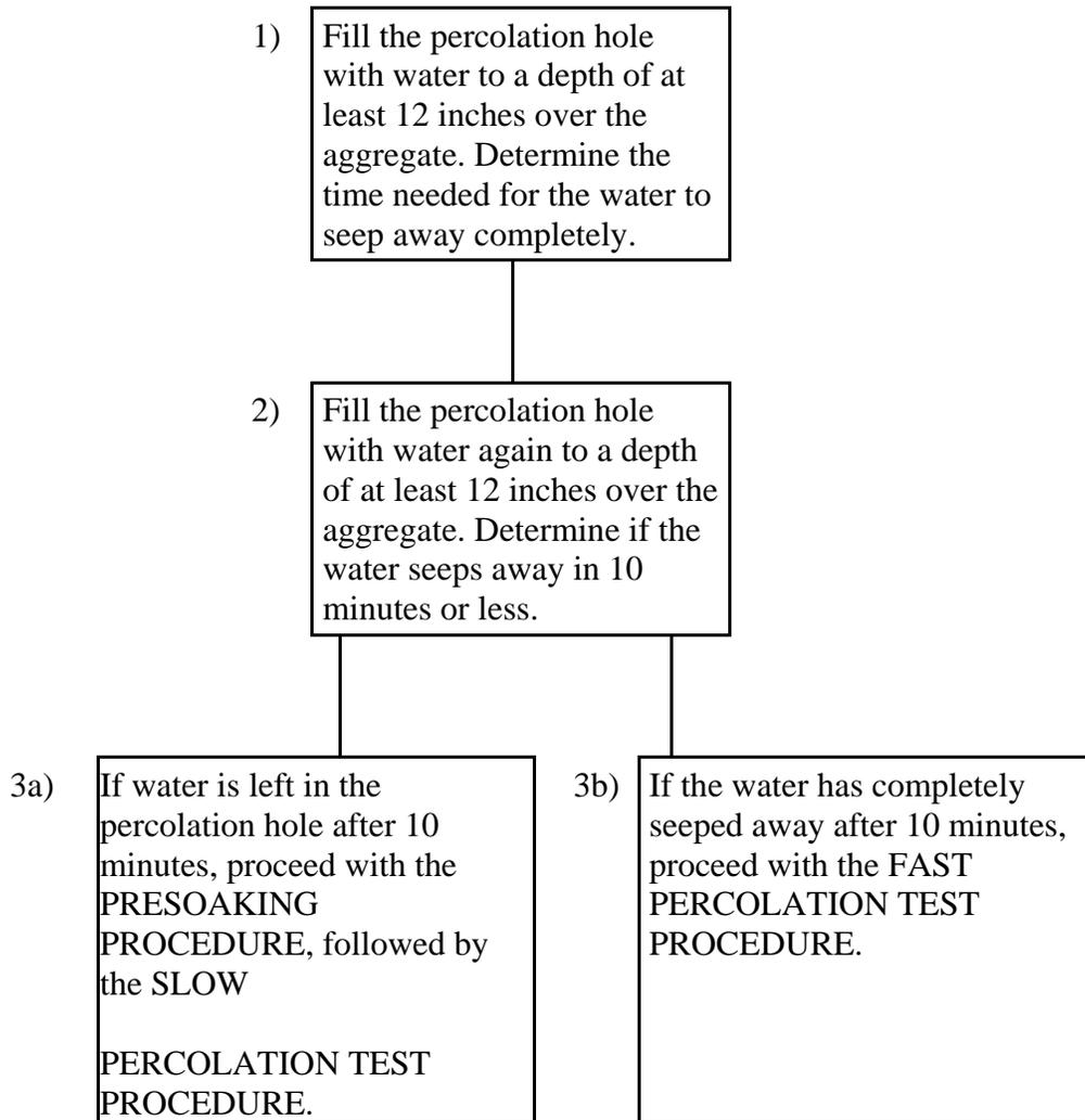
**NAC 444.7964 Fast percolation test procedure. (NRS 439.200, 444.650) The following flow chart illustrates the fast percolation test procedure:**
